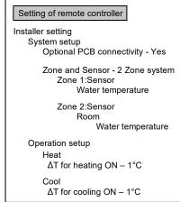
This is an example of simple 2 zone control without using buffer tank.
