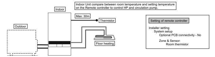
Connect floor heating or radiator directly to Indoor Unit.
