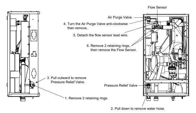
⚠ When reinstall Flow Switch, ensure the arrow on the flow switch is parallel with the pipe shaft and is facing in the direction of flow.
