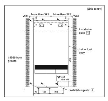
The centre of installation plate should be at more than 375 mm at right and left of the wall.
