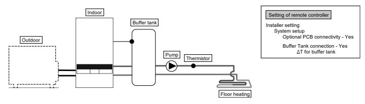
This is an application that connects the buffer tank to the Indoor Unit. Buffer tank's temperature is detected by buffer tank thermistor (specified by Panasonic). This system requires Optional PCB (CZ-NS5P).
