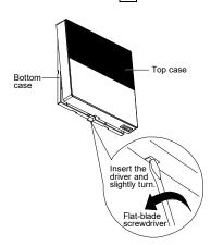
3. Reverse the steps 1 to 4 of section "Remove The Remote Controller From Indoor Unit" to fix Remote Controller Case 7 on Indoor Unit.
