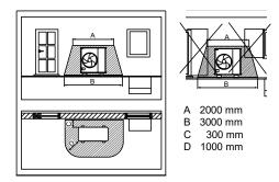
3) Protective zone for ground installation in a building corner
