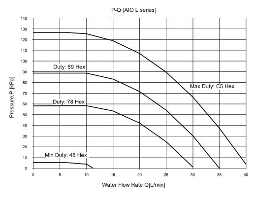
\* This condition is under connecting ODU and connecting 5m piping (inner diameter Φ25) between ODU and IDU (AIO).
