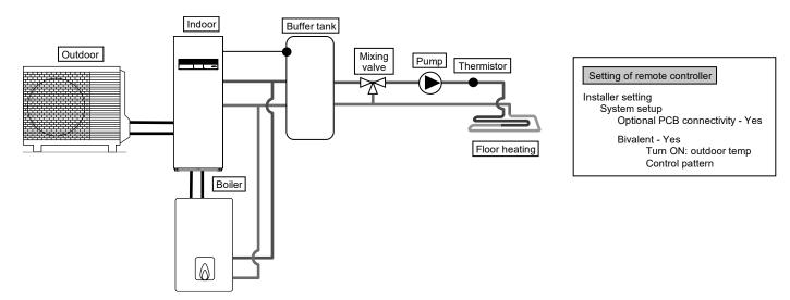
This is an application that connects the boiler to the Tank Unit, to compensate for insufficient capacity by operate boiler when outdoor temperature drops & heat pump capacity is insufficient.
