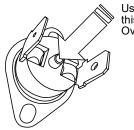
Use test pen to push this button for reset Overload protector ②.
