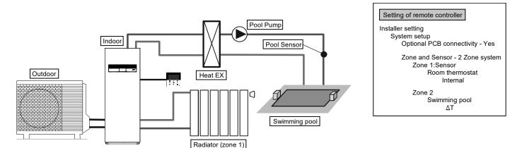
Connect floor heating and swimming pool to 2 circuits through buffer Tank Unit as shown in figure. Install additional pool heat exchanger, pool pump and pool sensor on pool circuit. Remove remote controller from Tank Unit and install in room where floor heating is installed. Circulation water temperature of floor heating and swimming pool can be set independently.
