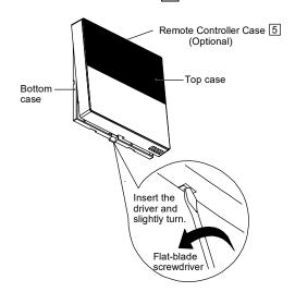
3. Reverse the steps 1 to 4 of section "Remove The Remote Controller From Tank Unit" to fix Remote Controller Case 5 on Tank Unit.
