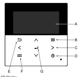
Name Function A: Main screen Display information Open/Close main menu B: Menu C: Triangle (Move) Select or change item D: Operate Start/Stop operation E: Back Back to previous item F: Quick Menu Open/Close Quick menu G: OK Confirm
