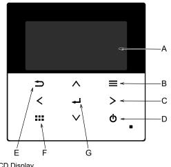
Name **Function** A: Main screen Display information Open/Close main menu B: Menu Select or change item C: Triangle (Move) D: Operate Start/Stop operation E: Back Back to previous item F: Quick Menu Open/Close Quick menu G: OK Confirm
