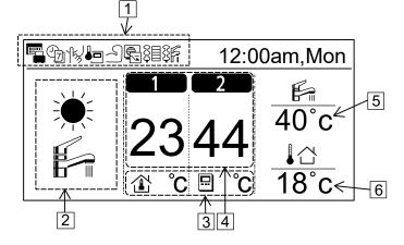
Function Name 1: Function icon Display set function/status Demand control Holiday mode Weekly timer Room heater Quiet mode Tank heater Remote controller room thermostat Powerful mode
