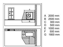
4) Protective zone for wall installation in front of a building wall
