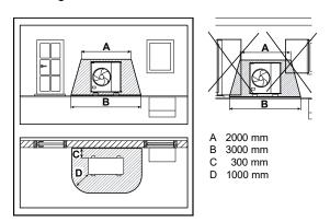
3) Protective zone for ground installation in a building corner
