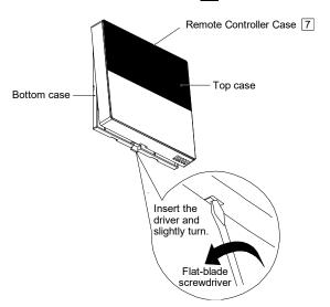
3. Reverse the steps 1 to 4 of section "Remove The Remote Controller From Indoor Unit" to fix Remote Controller Case 7 on Indoor Unit.
