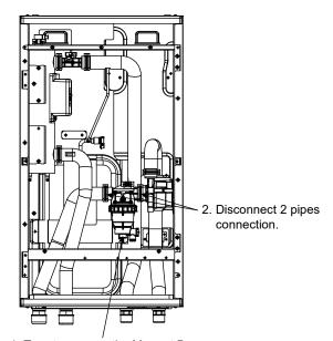
Turn to remove the Magnet Bar at bottom of Magnetic Water Filter Set.
