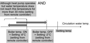
In Advanced Parallel mode, setting for both heating and tank can be made simultaneously. During operation of "Heating/Tank" mode, when each time the mode is switched, the boiler output will be reset to OFF. Please have good understanding on the boiler control characteristic in order to select the optimal setting for the system.
