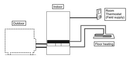
Setting of remote controller Installer setting System setup Optional PCB connectivity - No Zone & Sensor: Room thermostat (External)
