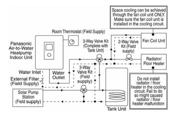
Diagram 4.1: Typical Water Piping Installation
