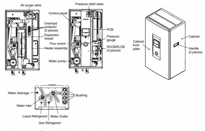
Water pump: The pump circulates the water in the water circuit.
