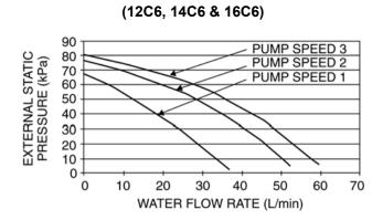
Flow rate characteristic of indoor unit is as per above mentioned.
