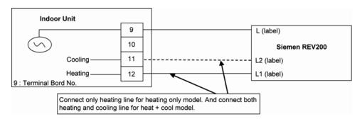
Wire Connection and thermo characteristic of Siemen RAA20:
