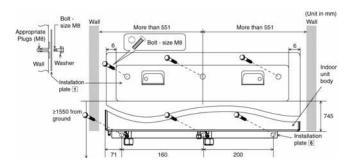
The centre of installation plate should be at more than 551 mm at right and left of the wall.
