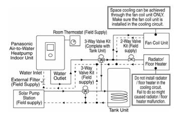
Diagram 4.1: Typical Water Piping Installation
