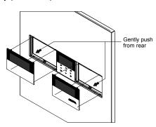
2. Remove the 4 screws and take out the holder with Remote Controller ③.
