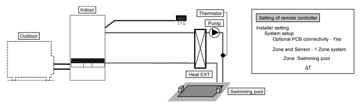
This is an application that connects to the swimming pool only. Connects pool heat exchanger directly to Indoor Unit without using buffer tank. Install pool pump and pool sensor (specified by Panasonic) at secondary side of the pool heat exchanger. Remove remote controller from Indoor Unit and install in room where floor heating is installed. Temperature of swimming pool can be set independently. This system requires the Optional PCB (CZ-NS5P).
