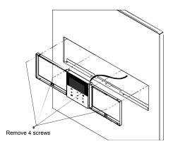
3. Remove the top case from the bottom case.
