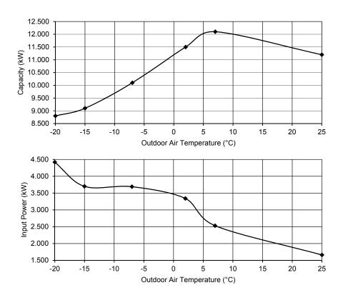
Condition Outdoor air temperature : 35°C (DBT), -°C (WBT) Indoor water inlet temperature : 12°C Indoor water outlet temperature : 7°C Piping length : 7 m
