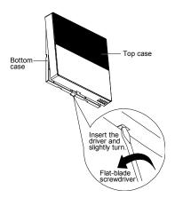
Reverse the steps 1 to 4 of section "Remove The Remote Controller From Indoor Unit" to fix Remote Controller Case 7 on Indoor Unit.
