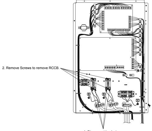
1. Disconnect lead wires.
