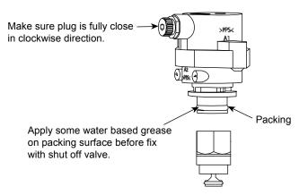
During reinstall Flow Sensor
