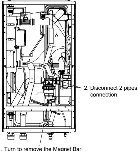
1. Turn to remove the Magnet Bar at bottom of Magnetic Water Filter Set.
