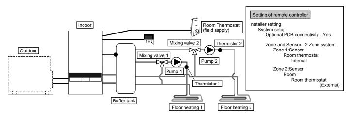
Connect floor heating to 2 circuits through buffer tank as shown in the figure.
