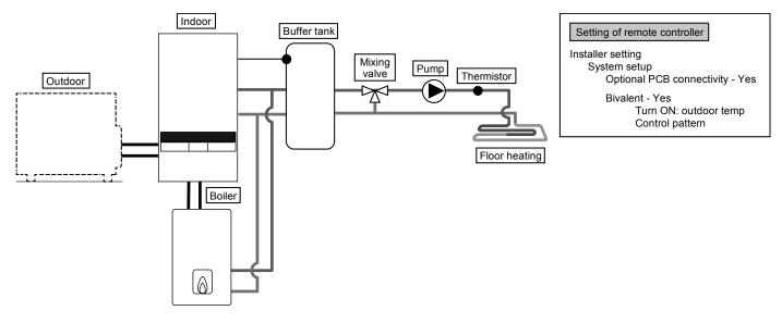
This is an application that connects the boiler to the Indoor Unit, to compensate for insufficient capacity by operate boiler when outdoor temperature drops & heat pump capacity is insufficient.
