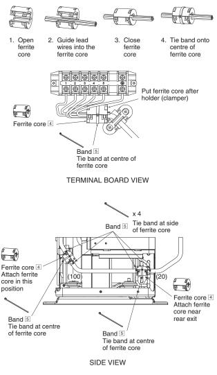
DETAIL OF FERRITE CORE INSTALLATION
