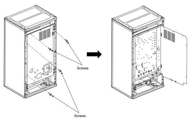
1. Remove 4 screws from the Control Board Cover.
