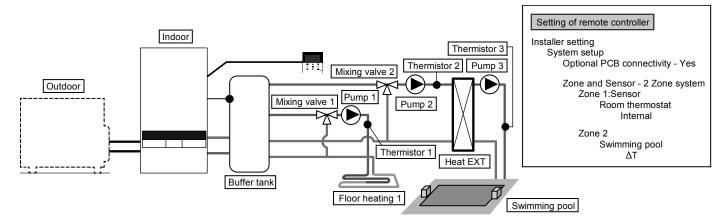
Connect floor heating and swimming pool to 2 circuits through buffer tank as shown in figure.
