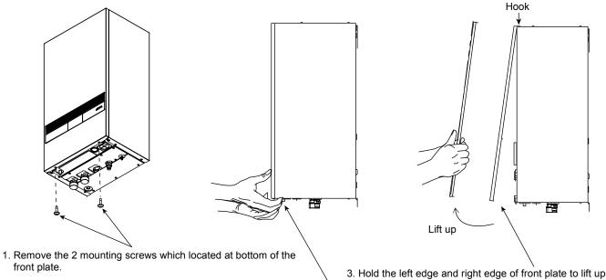
3. Hold the left edge and right edge of front plate to lift up front plate from hooks.
