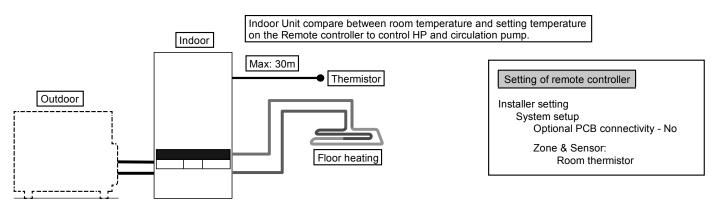
Connect floor heating or radiator directly to Indoor Unit. Remote controller is installed on Indoor Unit.
