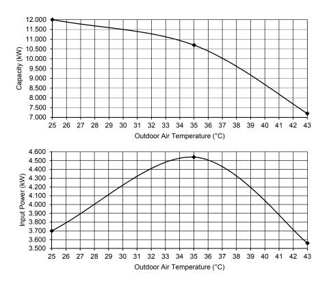
Condition Outdoor air temperature : 35°C (DBT), -°C (WBT) Indoor water inlet temperature : 23°C Indoor water outlet temperature : 18°C Piping length : 7 m
