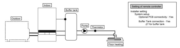
This is an application that connects the buffer tank to the Indoor Unit.
