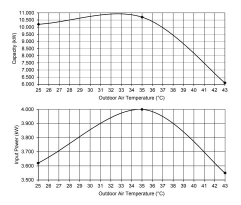
Condition Outdoor air temperature : 35°C (DBT), -°C (WBT) Indoor water inlet temperature : 19°C Indoor water outlet temperature : 14°C Piping length : 7 m
