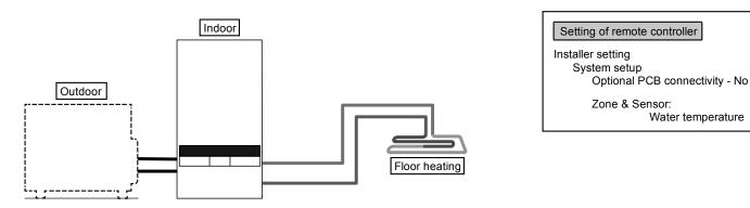
Connect floor heating or radiator directly to the Indoor Unit. Remote controller is installed on Indoor Unit. This is the basic form of the most simple system.
