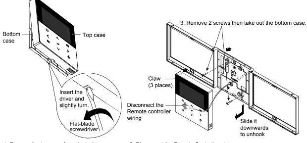
1. Remove the top case from the bottom case.
