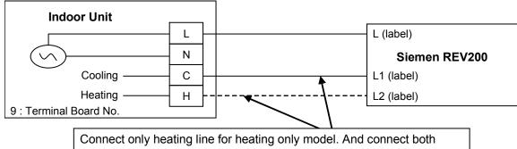
heating and cooling line for heat + cool model.
