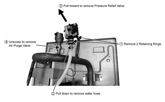
$\triangle$  When reinstall the water pipe, use grease or water at the joining.
