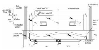
The centre of installation plate should be at more than 551 mm at right and left of the wall.
