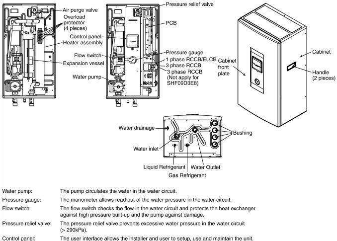
Control panel:The user interface allows the installer and user to setup, use and maintain the unit.Electric Heater:Additional heating capacity to the system when water and ambient temp is low.Expansion Vessel:Storage for excessive water.
