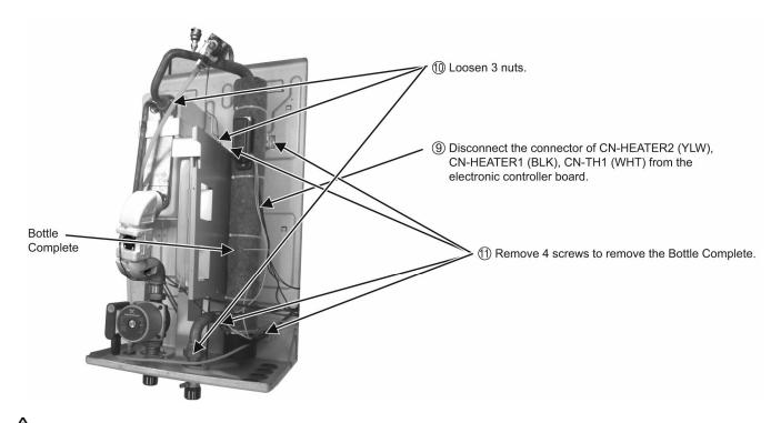
igtarrow When reinstall the water pipe, use grease or water at the joining.
