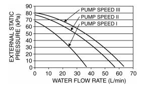
• Flow rate characteristic of indoor unit is as per above mentioned.
