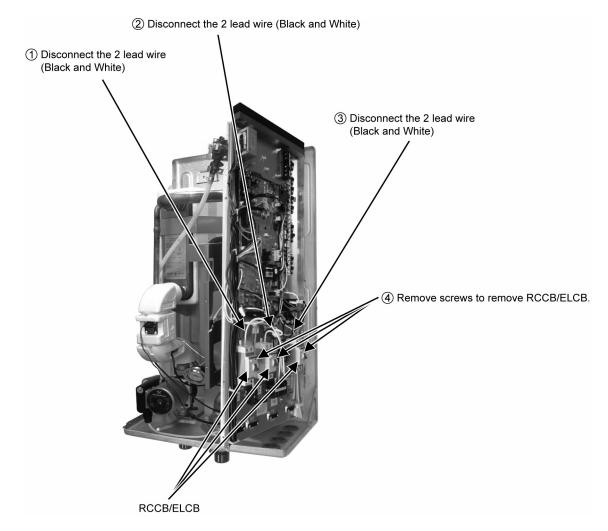
17.6 To Remove Transformer and Electronic Controller Board
