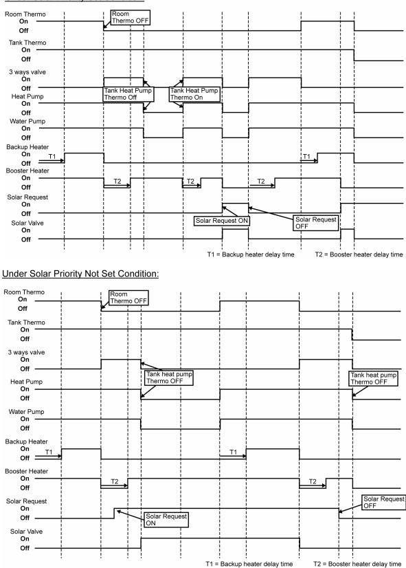
Setting 2: When heating priority is not set by control panel:
