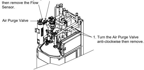
Mhen reinstall Flow Switch, ensure the arrow on the flow switch is parallel with the pipe shaft and is facing in the direction of flow.
