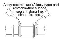
Neutral cure (Alkoxy type) & ammonia-free silicone sealant is only to be applied after pressure testing and cleaning up by following instructions of sealant, only to the outside of the connection. The aim is to prevent moisture from entering the connection joint and possible occurrence of freezing. Curing sealant will take some time. Make sure sealant will not peel off when wrapping the insulation.
